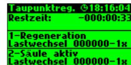
When daily checks are carried out, be mindful of any noises which are caused by the regeneration process. The pressure gauges should also be taken into consideration here. The expansion and noises of the purging air should always be regular. Brief interruptions in the flow noises for example indicate a defective solenoid valve or control fault.
