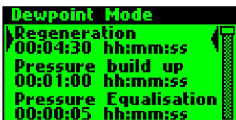
You can only change the cycle times using a password. This applies to all cycle times of the individual operating modes.
