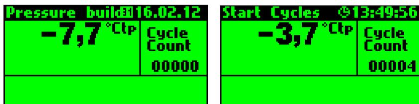
Under Anzahl Zyklen (Number of cycles), all cycles are counted which have been run in the current mode since startup.
