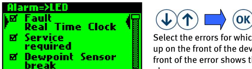
Select the errors for which the LED should light up on the front of the device. The checkmark in front of the error shows the activation of the alarm.
