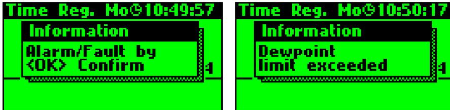
By pressing the **OK** key, you can hide the message for 2 minutes, but the alarm remains in the potential-free output and alarm LED.
